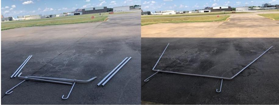
Tap the bottom pieces into the ground with the stakes in two places.....use a rubber mallet. You will see where the stakes go to hold it onto the ground. Put the other poles on top of the bottom pieces where they are swaged and crimped. Each side will have two poles. Angle the launcher so it is directly into the wind. You will put the poles away from the shore (rotate on stakes) and they lay on the ground. The whole apparatus swivels on the stakes.
